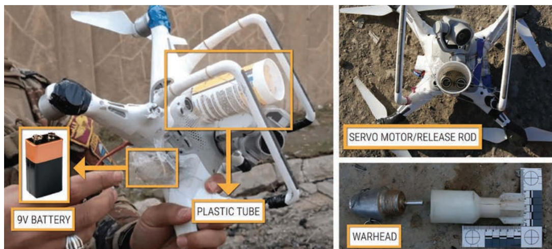
The Islamic State weapons system employed cheap quadcopter drones and fixed-wing drone platforms. These photographs, for example, show a commercial drone modified for projectile drop capability by Islamic State operatives. Credit: Don Rassler, Combating Terrorism Center at West Point U.S. Military Academy (Photos: Mitch Utterback and Conflict Armament Research)
