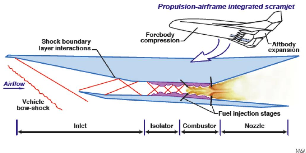
Instead of using a rotating compressor like a turbojet engine, the scramjet relies on forward velocity and aerodynamics to compress air into the engine before hydrogen fuel is introduced and subsequently combusted. It is, in effect, an "air breathing" technology with no moving parts. Whereas a ramjet decelerates the air to subsonic velocities before combustion, the airflow in a scramjet is supersonic throughout the entire engine.
