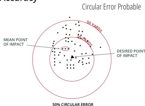
Each of the three main kinds of accuracy errors for ballistic, cruise, and hypersonic missiles has a different solution. Aim-point (targeting) and launch errors can be solved by greater diligence in surveying methods. Guidance errors, which occur while a vehicle is in flight, are measured by a missile's circular error of probability (CEP) and deviation of the mean impact point from the actual aim point. These errors are typically resolved by iterative tests and design corrections.
