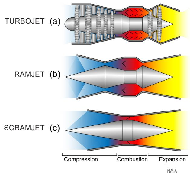
Figure: How scramjets work
