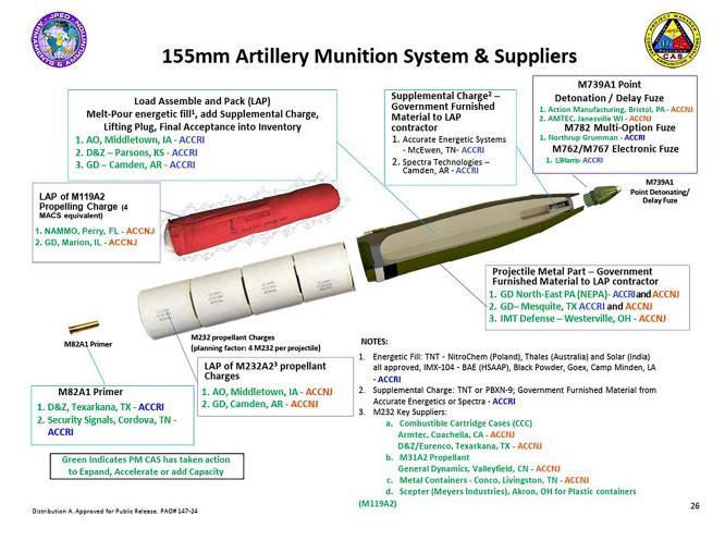
Diagram of 155mm munition system and suppliers. Four individual propellant charges are pictured behind the projectile. Image accessed via the US Army's Joint Program Executive Office (IPEO) for Armaments and Ammunition.
