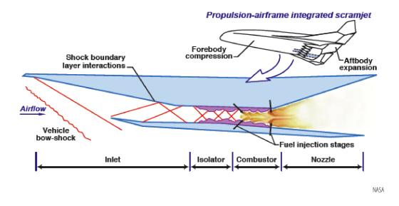
Instead of using a rotating compressor like a turbojet engine, the scramjet relies on forward velocity and aerodynamics to compress air into the engine before hydrogen fuel is introduced and subsequently combusted. It is, in effect, an "air breathing" technology with no moving parts. Whereas a ramjet decelerates the air to subsonic velocities before combustion, the airflow in a scramjet is supersonic throughout the entire engine.
