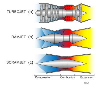
Figure: How scramjets work
