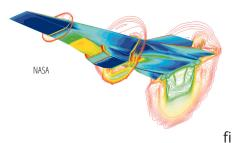
The enormous amount of thrust and speed generated by scramjets produce air friction and intense heat from molecular dissociation, imposing constraints on system design and materials. Hypersonic technology must be composed of materials that can withstand temperatures of up to 2200 degrees Celsius. Woven silicon carbide (SiC, very similar to carbon fibre), coupled with an oxygen-resistant ceramic coating, is currently one of the best available options for thermal
