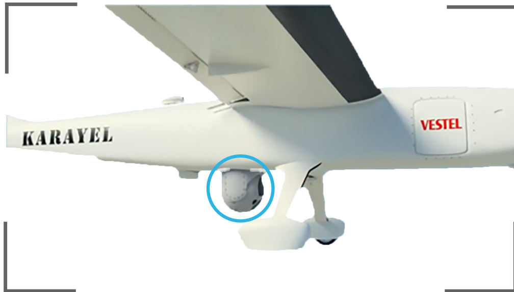
Fig. 6: Vestel Karayel UAV with MX-15D visible on the underside. Adapted screenshot from Vestel Defence Industries promotional video. 38
