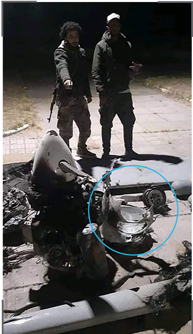
Fig. 14: Amended image of wreckage from reports of a Turkish-flown TB2 downed in Tarhouna, Libya, April 2020. Inverted housing of MX-15D visible in the debris. 90
