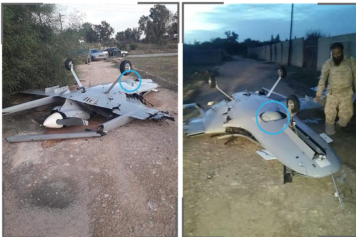
Fig. 13: Amended image of downed TB2 reportedly supplied to the GNA outside of Tripoli, December 2019. MX-15D visible in underside of the vehicle. 83
