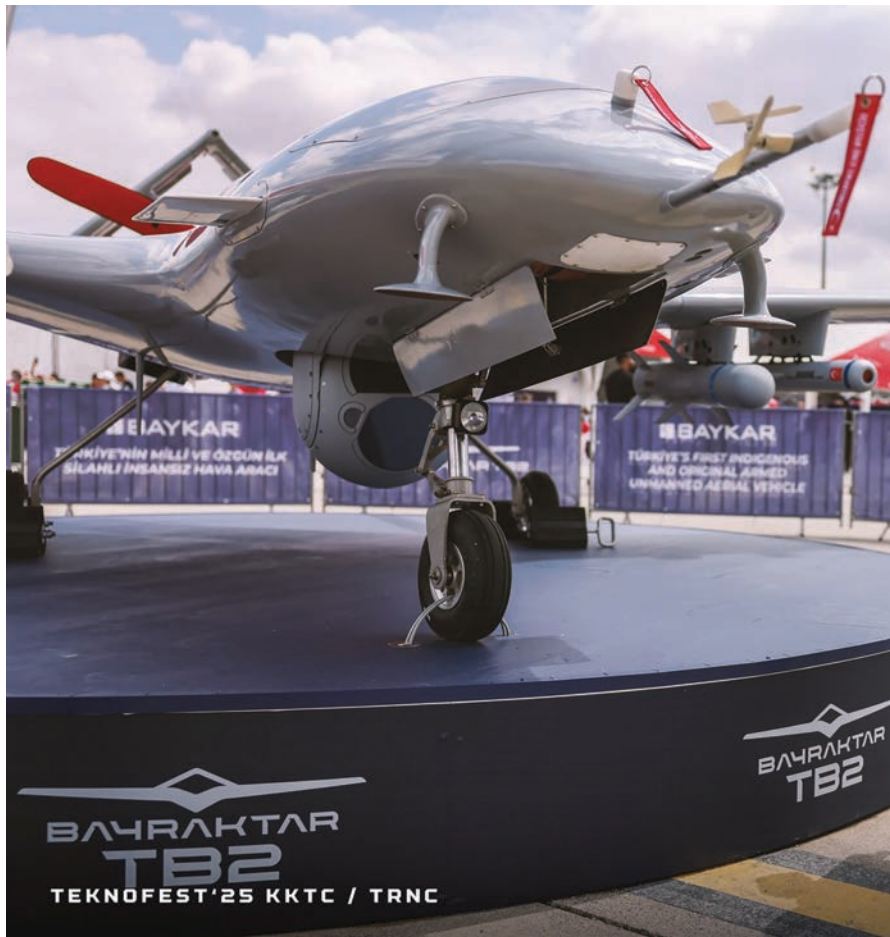
Bayraktar TB2 UAV pictured with a L3Harris Wescam CMX-15D EO/IR sensor visible on its underside during Teknofest 2025, May 2025. It is unclear when this sensor unit was exported to Türkiye. Photo: Baykar
